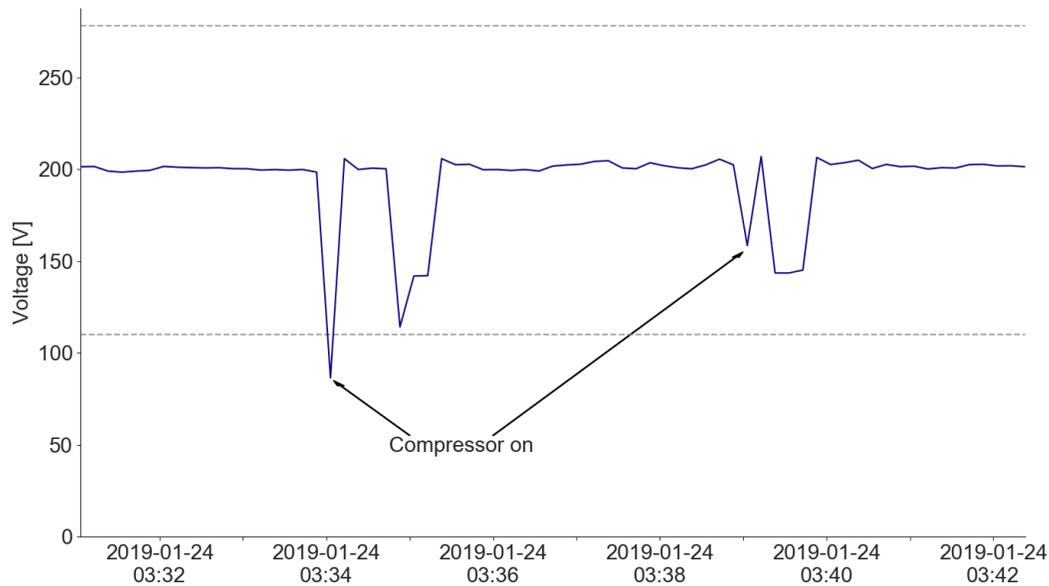
Figure 22: High source impedance, device K-080.
