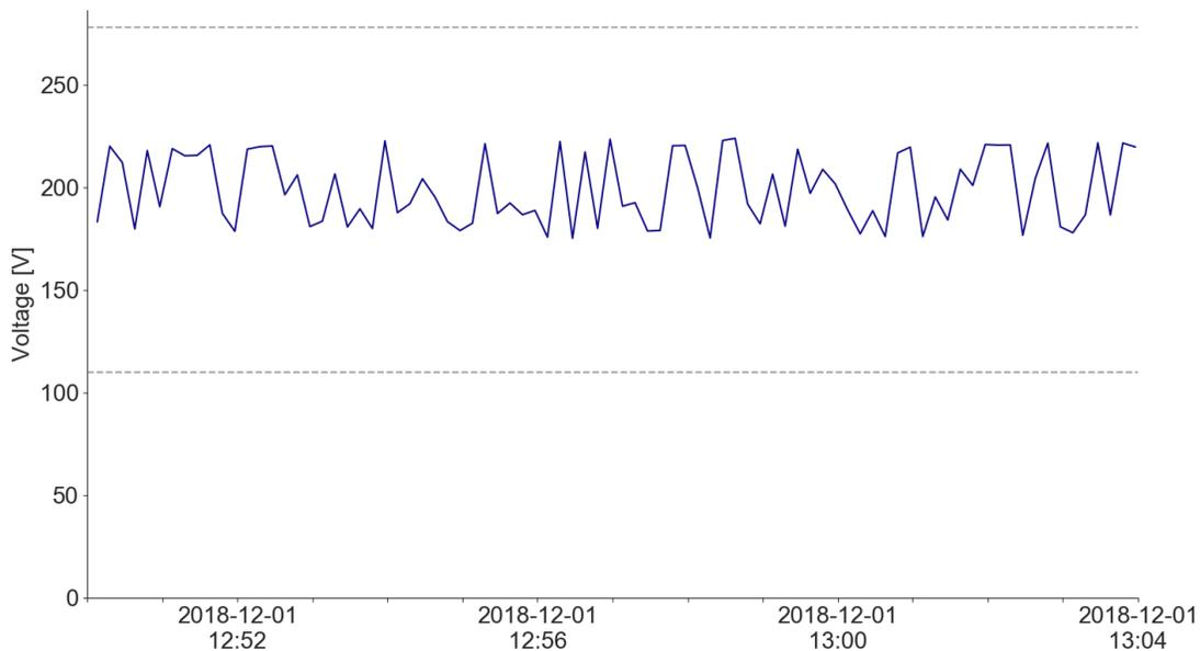
*Figure 21: Transient undervoltage conditions in Kenya, expanded view of previous figure. Note the 50 V jumps and drops from one 10-second interval to the next.*
