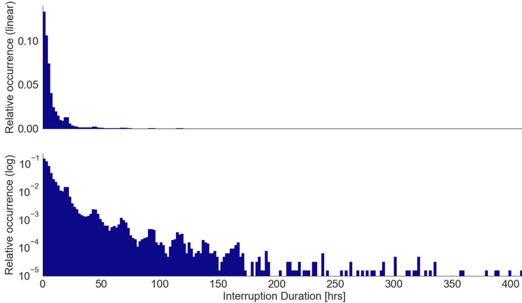
Figure 11: Interruptions greater than 30 minutes in Nigeria, as reported by devices during the study period. Upper graph shows the relative fraction of occurrences on a linear scale; the lower graph shows them on a logarithmic scale. Bin width is set to 2 hours.
