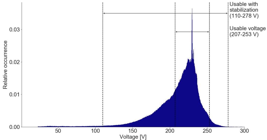
Figure 16: Line voltages reported by devices in Nigerian facilities during the study period (normalized to 1). Each x-axis bin represents 0.1 V. Mean is 209.9 V; standard deviation is 33.5 V.
