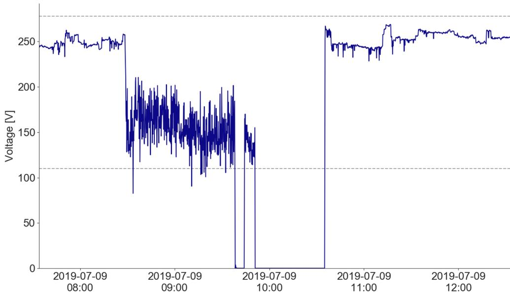
Figure 37: Variable voltage mostly within the stabilizable range, device K-154.
