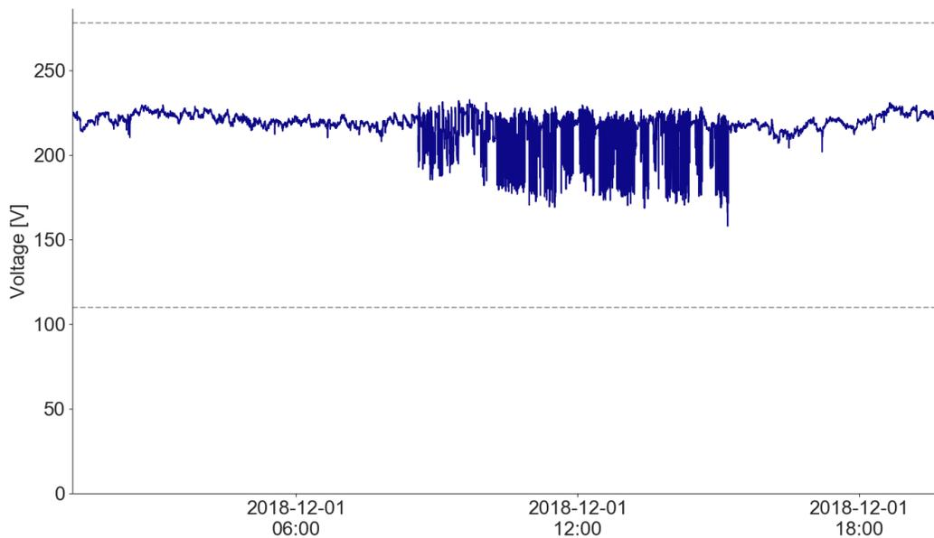
Figure 20: Transient undervoltage conditions in Kenya. During this multi-hour period, reported line voltage occasionally spiked by 50 V during 10-second intervals. An expanded view is shown in Figure 21. Device is K-172.
