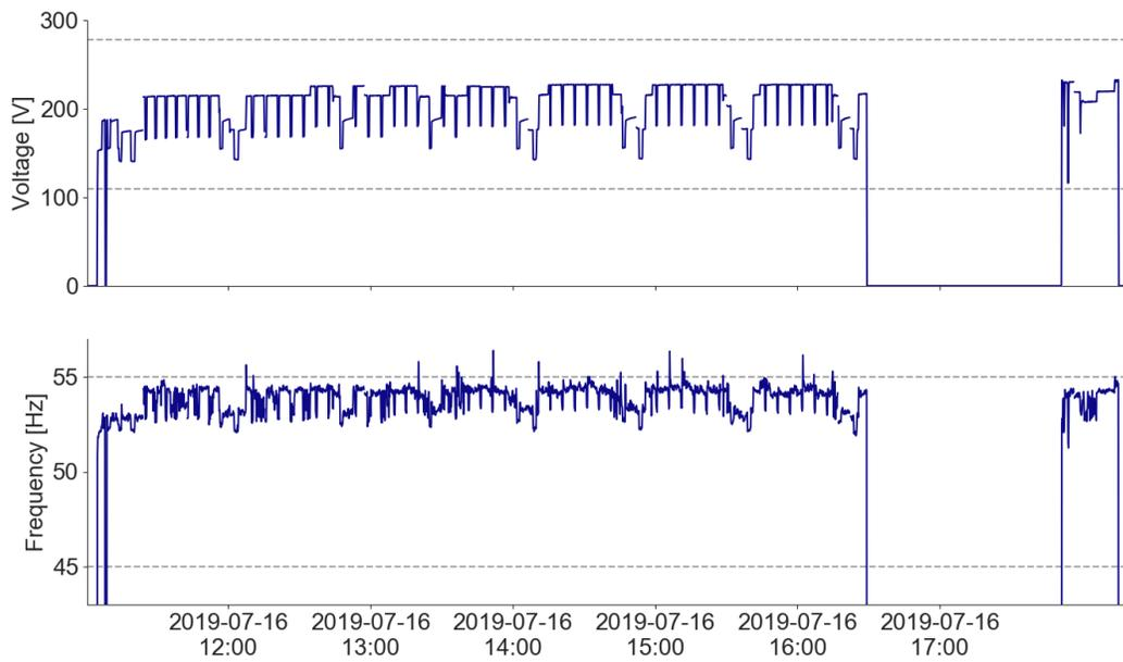
Figure 46: Voltage and frequency varying with load, device N-060.
