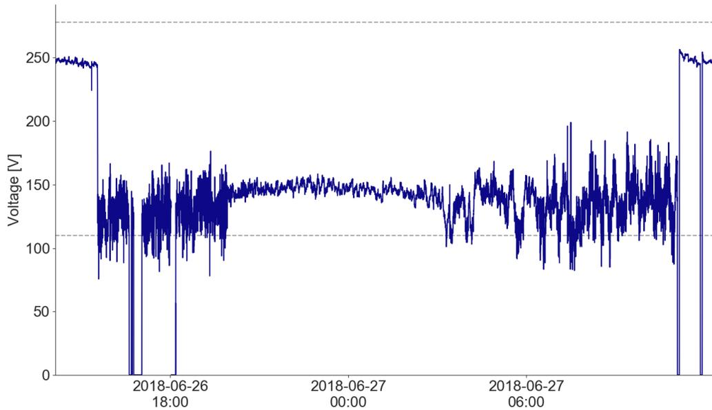
*Figure 18: Sustained undervoltage in Kenya, device K-147.*
