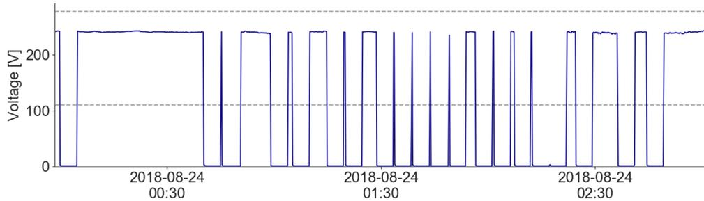
Figure 14: Time series plot of voltage reported by a device in a Kenyan facility. The voltage range usable with stabilization is between the horizontal dashed lines. Device K-026.
