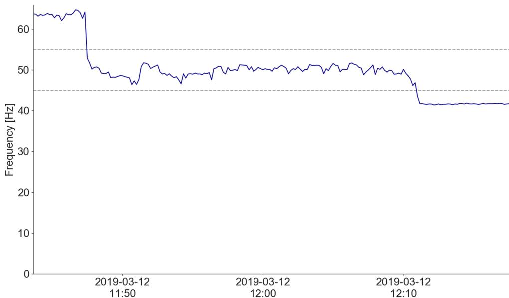
Figure 25: Generator frequency dropping under load. Horizontal dashed lines at 45 Hz and 55 Hz. Device is N-089.
