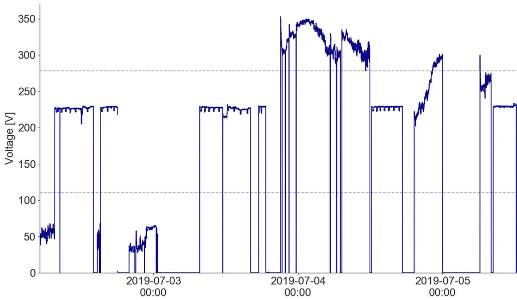
Figure 41: Usable voltage, overvoltage, undervoltage, and zero voltage over a 3-day period, device N-044.
