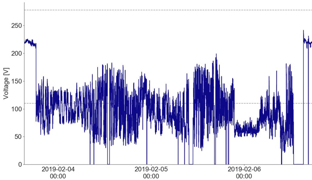
Figure 19: Highly transient undervoltage conditions in Nigeria, device N-058.
