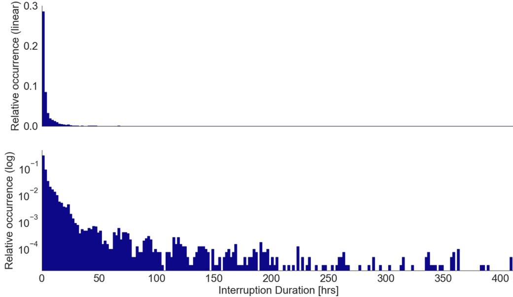
Figure 10: Interruptions greater than 30 minutes in Kenya, as reported by devices during the study period. Upper graph shows the relative fraction of occurrences on a linear scale; the lower graph shows them on a logarithmic scale. Bin width is set to 2 hours.
