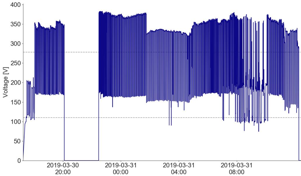
Figure 44: Square wave stepping between stabilizable undervoltage and unstabilizable overvoltage. The pattern is roughly periodic every 3-4 minutes, device N-070.
