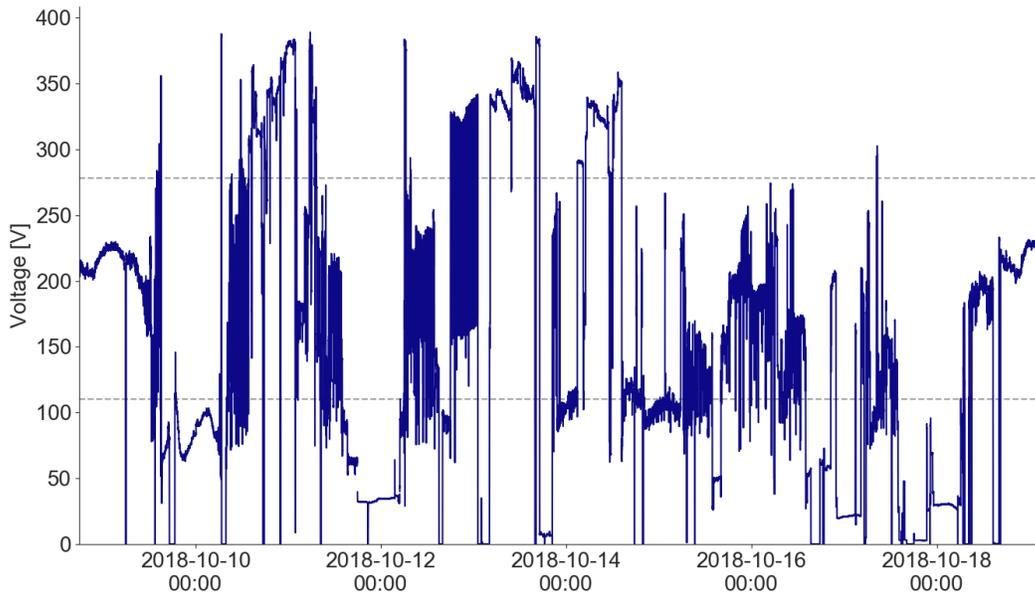
Figure 36: Variable voltage including overvoltage, device N-048.
