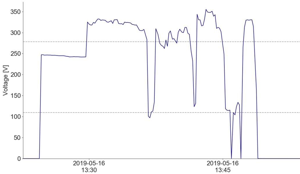
Figure 42: Undervoltage to overvoltage several times within a 15-minute span, device N-082.
