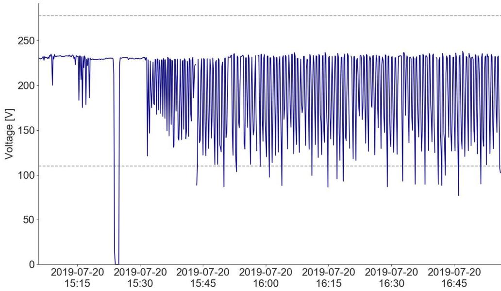
Figure 40: Rapid fluctuations, device N-054.
